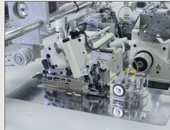
Contour guide, photo cell and sewing head form an optimal unit
