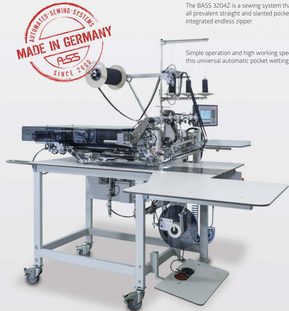
The BASS 3204Z is a sewing system that can process all prevalent straight and slanted pocket openings with integrated endless zipper.
