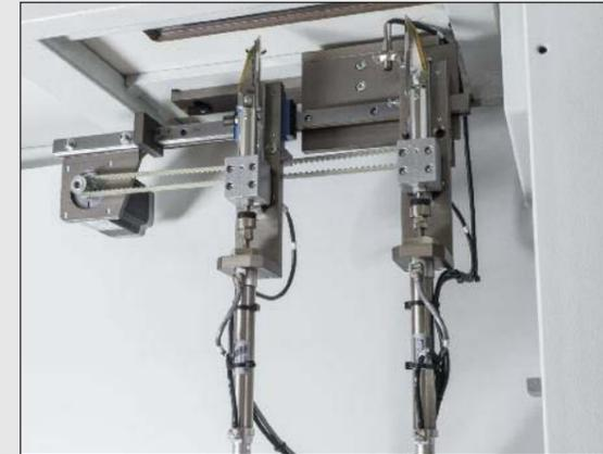
Cutter block with stepper motor drive
