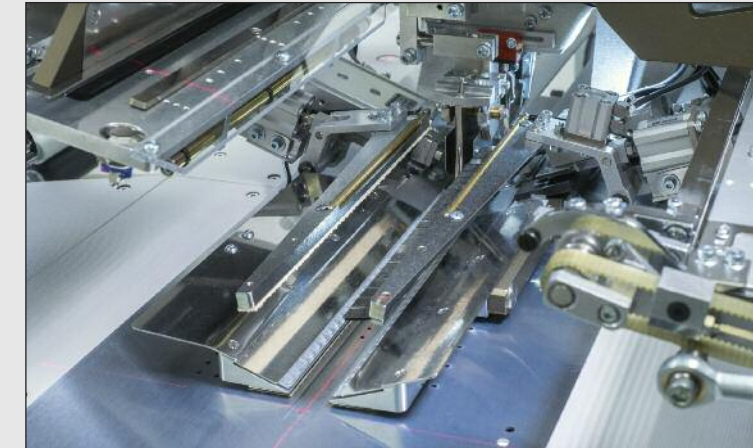
Automatic transfer unit for piping and accessories
