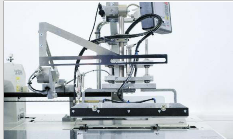
Folder for holding and positioning borders and fly pieces
