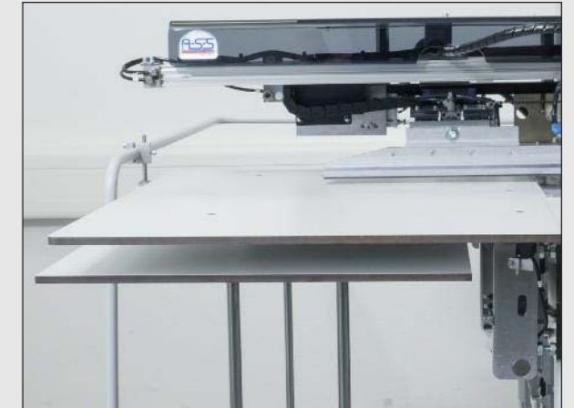
Automatic stacker for pocket pouches
