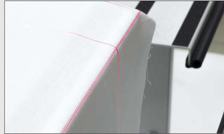
Positioning of the sewing part on the marking lights of the pre-laying station
