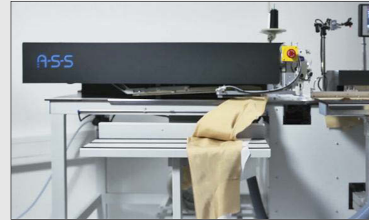
Automatic de-stacking of the sewed parts
