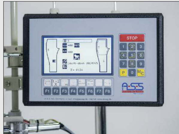
Easy administration and retrieval of the programmed seams via the program controller
