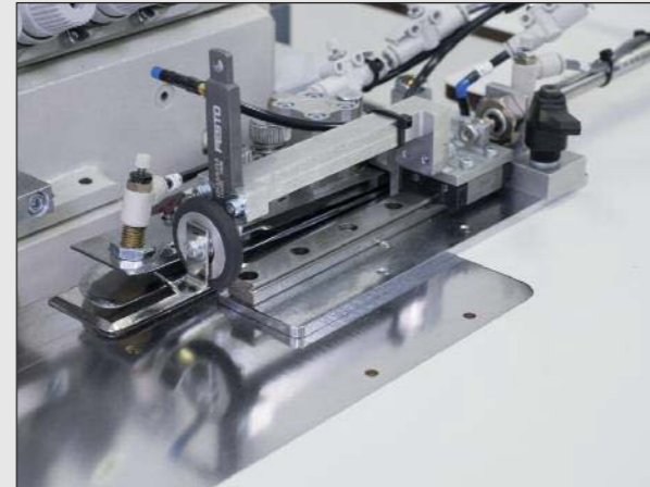
The accurately adjustable contour guide ensures consistent seam widths over the entire seam length even with seam interruption
