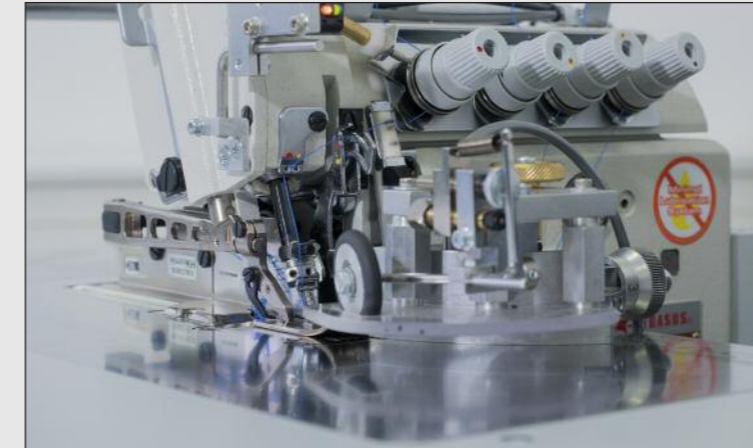
The optimal unit for sewing work: Contour guide, photocell and sewing head.
