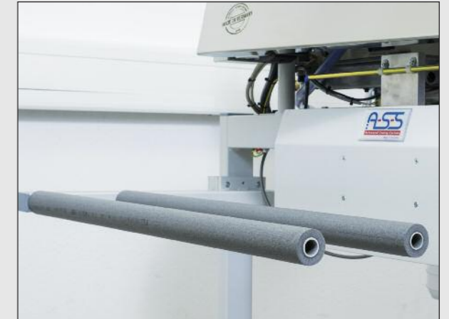
The exact and fast working stacker unit deposits the sewing parts for further processing.
