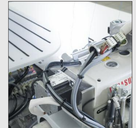
Stepper motor-controlled differential and top transport
