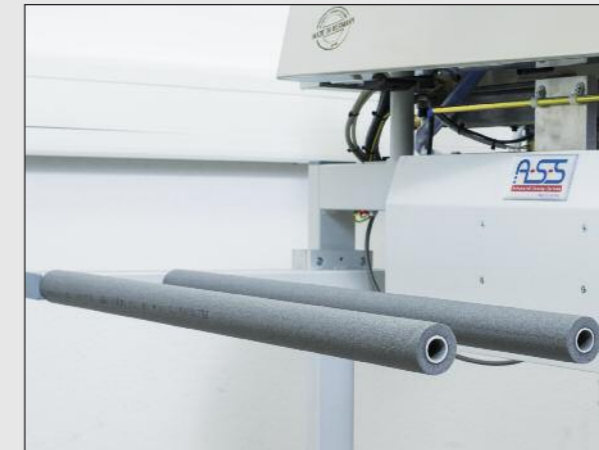
The exact and fast working stacker unit deposits the sewing parts for further processing.
