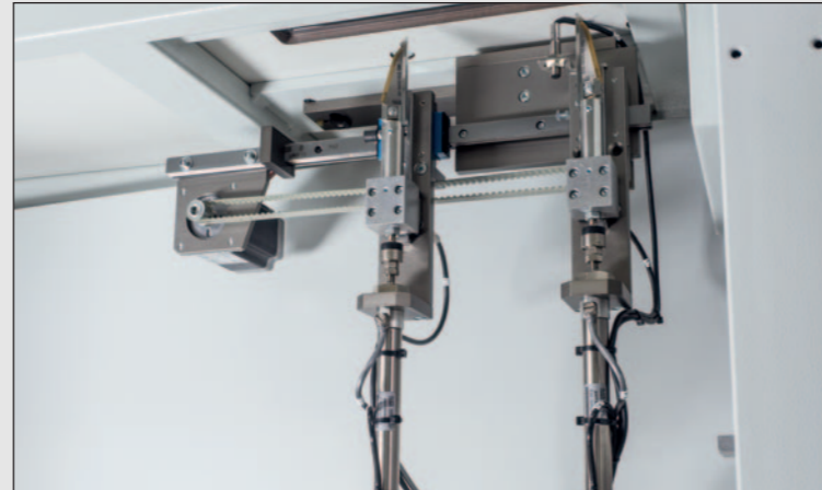
Cutter block with stepper motor drive
