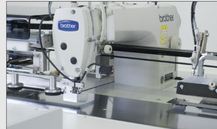
Seam length detection by the photo cell
