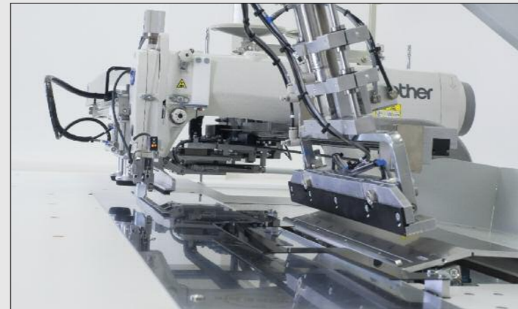
After placing the pocket pouch and laying the border, the machine performs the following work steps such as in-feed, sewing operation and de-stacking automatically.
