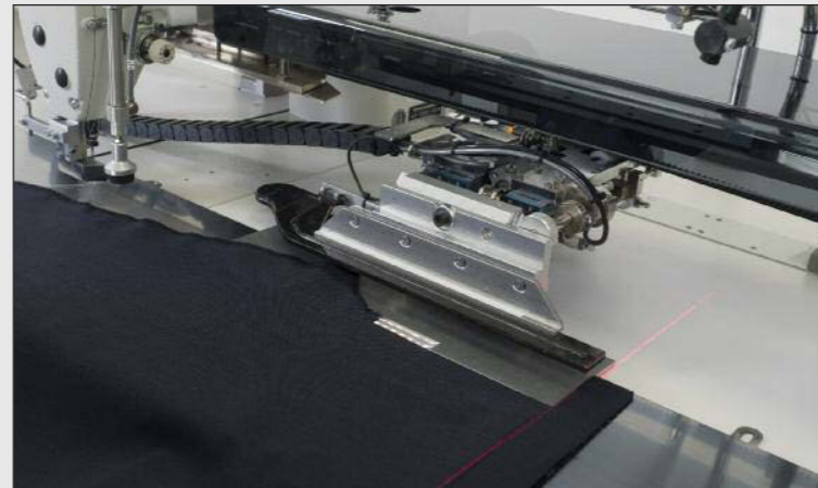
The sewing item positioned exactly in advance by the operator is accepted by the transport clamp
