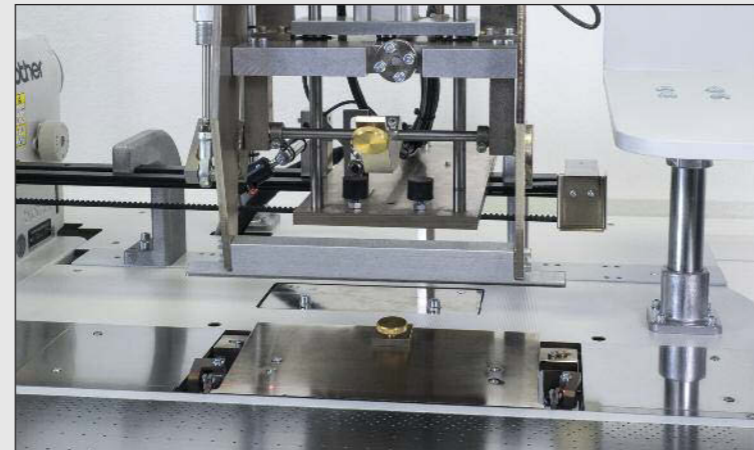
With the help of the model-specific markings, the sewing material can be positioned accurately for the subsequent sewing process
