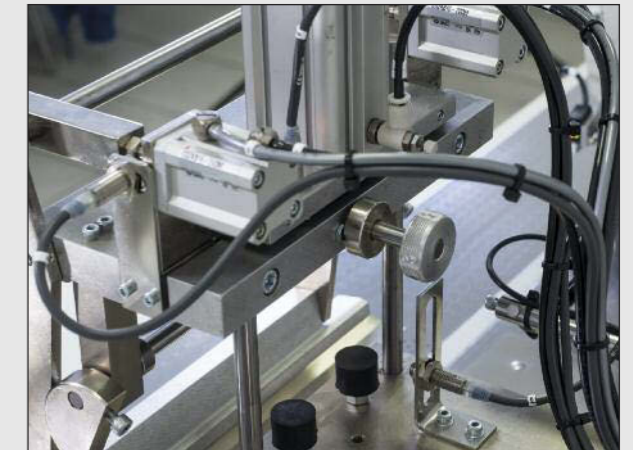
The top-stitch widths are adjusted mechanically
