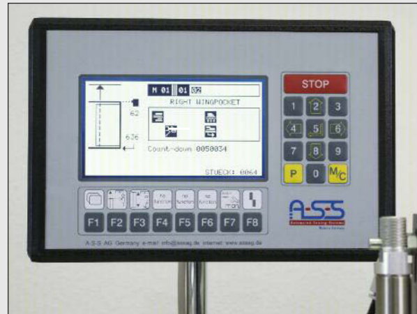
Easy administration and retrieval of the pre-programmed seams and seam widths
